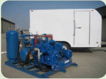
200 cubic meter / hr pilot unit blower, compressor and after cooler
