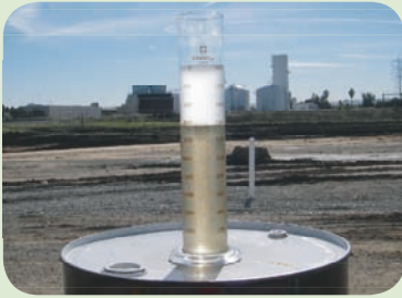
Graduated cylinder with DNAPL underlying water condensate
