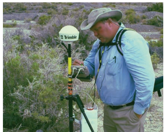
(Top) Willowstick operator prepares electrode antenna wire prior to energizing the survey area. (Bottom) Willowstick operator collects magnetic field readings using the AquaTrack instrument. The instrument detects magnetic fields using specialized, highly sensitive magnetic coils
